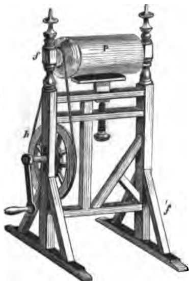
Fig. 73. Franklin's Electrical Machine.
